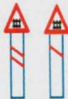
GUARDED LEVEL CROSSING
